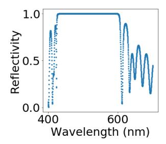
Figure 6: The normalised reflected flux for 16 bilayers with high  $(n_{\rm h} = 2.4)$  and low  $(n_{\rm l} = 1.4)$  index (quarter-wave at  $\lambda = 500$  nm) on a glass substrate. The result is a **high-reflectivity mirror**. Calculated by solving the linear eqns (21)-(26) numerically, see python notebook multilayer.ipynb online.
