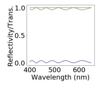
Figure 4: The normalised reflected (blue) and transmitted (green) flux for a 2  $\mu$ m thick layer with  $n_1^2 = n_0 n_2$ , where  $n_0 = 1.0$  and  $n_2 = 1.5$ , calculated using the Fabry Perot results, eqs (1) and (2). The orange curve shows that the total flux is conserved. The purple dots are calculated by solving the matrix equation, see python notebook multilayer.ipynb online.
