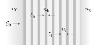
Figure 5: Schematic of a high-reflectivity mirror with alternating quarter-wave layers with high  $n_{\rm h}$  and low  $n_{\rm l}$  index. The quarterwave condition for the central wavelength  $\lambda_{\rm c}$ fixes the thickness of each layer, i.e.,  $\ell_{\rm h} = \lambda_{\rm c}/(4n_{\rm h})$  and  $\ell_{\rm l} = \lambda_{\rm c}/(4n_{\rm l})$ .
