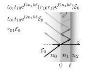
Figure 1: Thin film reflection. The first three contributions to the reflection coefficient are shown. Thereafter each subsequent term picks up another factor of  $r_{10}r_{12}e^{i2n_1k\ell}$ .
